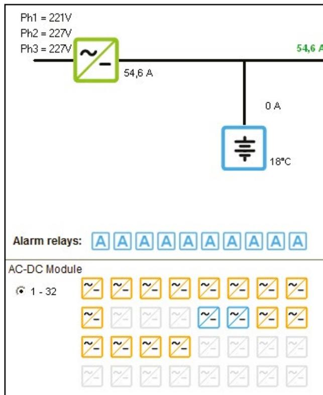
Figure 5 - PowCom™ window: Energy Saving in operation
