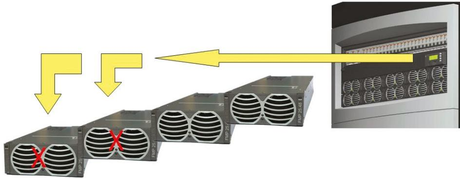
Figure 2 - ACC controls the operation of rectifiers
