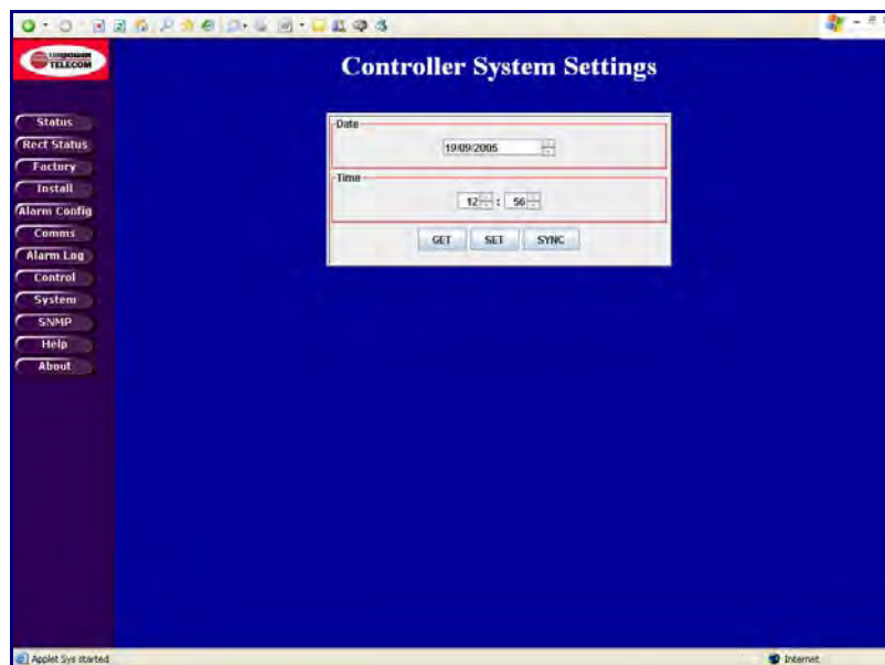
Figure 17 - Controller System Settings WEB Page (typical)
