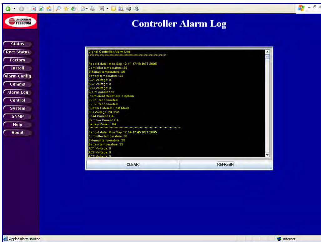
Figure 15 - Controller Alarm Log WEB Page (typical)
