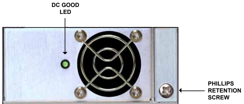
Figure 2. Front Panel of the Front End/Rectifier
